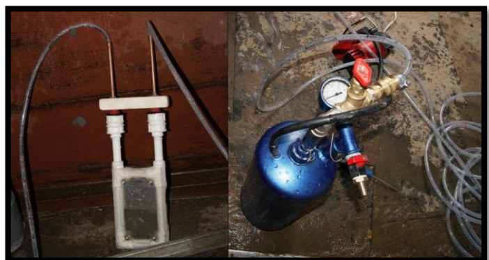
Fig.10 Tank flushing device
