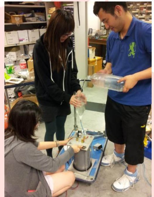
Fig. 39 Using the self-made pressurized tube to test the modules
