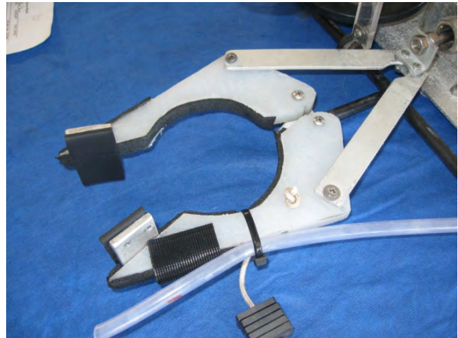
FIGURE 13 - FINISHED CLAW WITH MAGNET ATTACHED.
