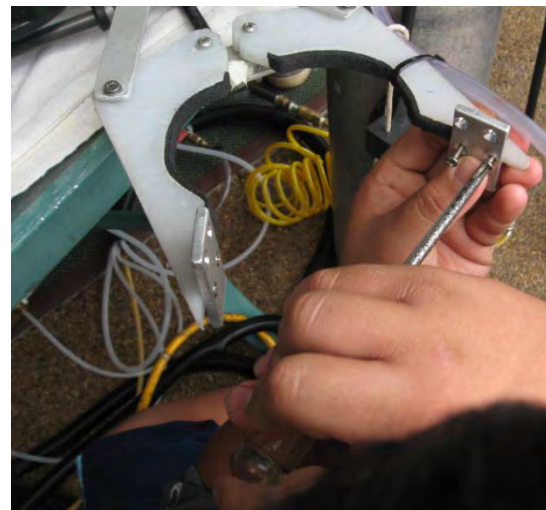
FIGURE 12 - INSTALLATION OF THE ALUMINUM METAL PANELS.
