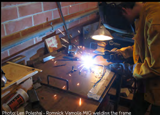
Photo: Len Poleshaj - Romnick Vamolja MIG welding the frame
