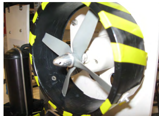
FIGURES 4 & 5- THE RIGHT BTD 150 HORIZONTAL THRUSTER (TOP) AND THE 380/500 BILGE PUMP LATERAL MOTOR (BOTTOM).
