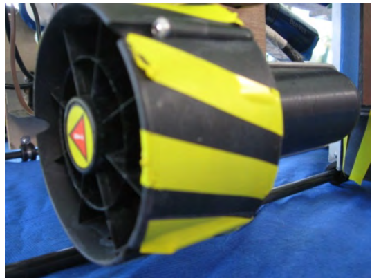
FIGURES 4 & 5- THE RIGHT BTD 150 HORIZONTAL THRUSTER (TOP) AND THE 380/500 BILGE PUMP LATERAL MOTOR (BOTTOM).
