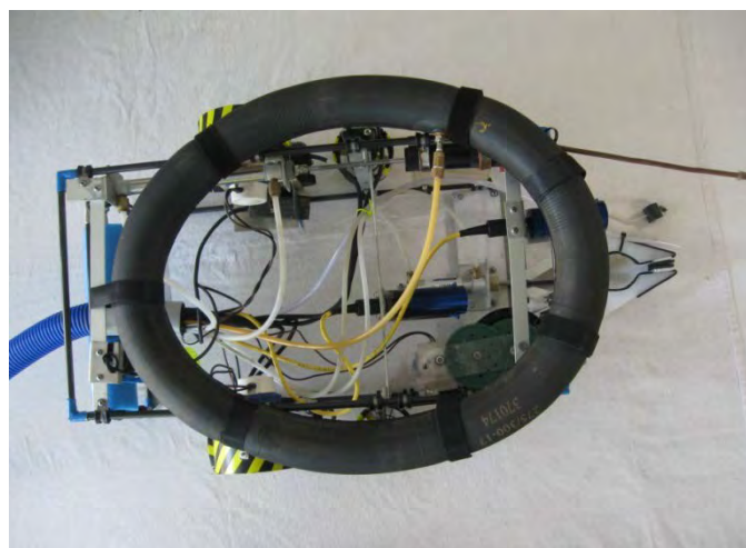
FIGURE 7 - FLOTATION BAG MOUNTED ON TOP OF C-LION
