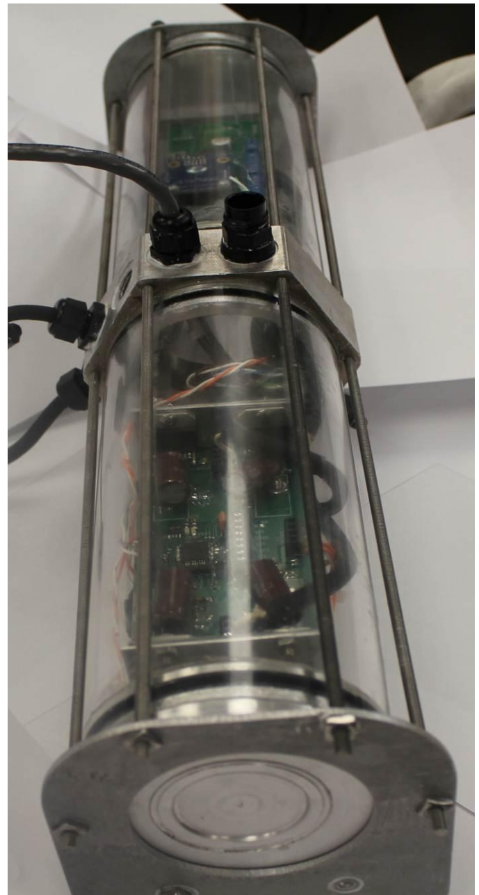
FIGURE 6 - SEALED ELECTRONICS HOUSING
