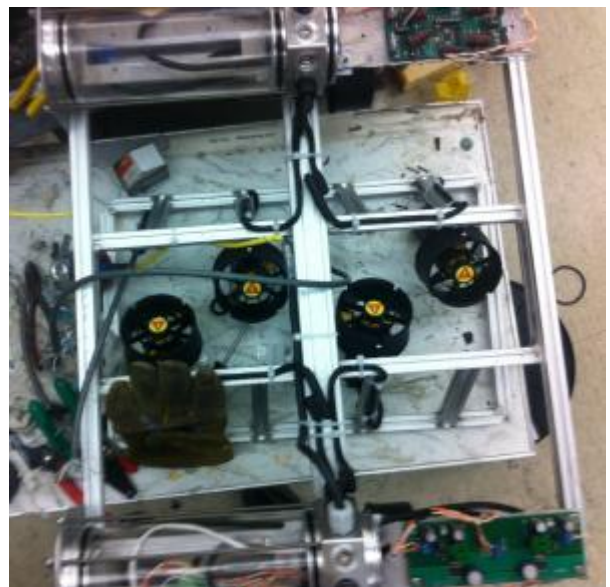
FIGURE 7 - VERTICAL VECTORED THRUSTERS
