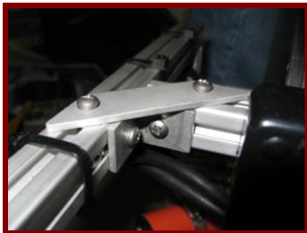
Figure 4: ROV Frame braces
