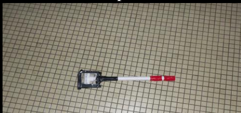
The ultrasonic thickness gauge sensor and the neutron back scatter device
