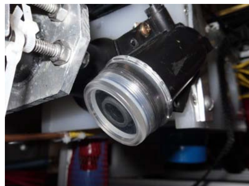
Figure 12. Camera is positioned directly at the gripper
