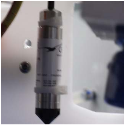
Figure 17. Keller depth sensor
