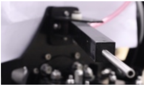
Fig. 7 - Oil Sampling Assembly with Sampling Rod Extended
