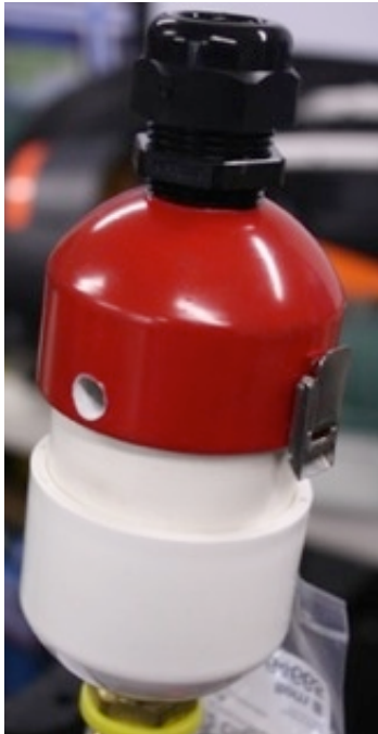
Fig. 12 - Tether Interconnect for Detachability
