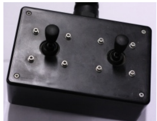
Fig. 10 - Joystick Controller That Utilize the ROV's Four Degrees of Freedom
