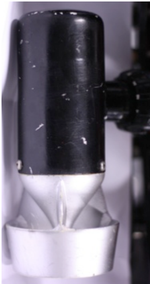
Fig. 5 - Team Made Bilge Pump Thruster
