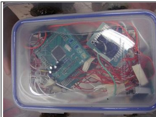
Underwater control box (Double layers of Lock and Lock boxes)
