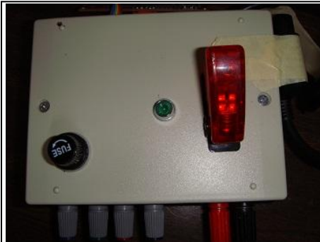
Onshore main control system (Arduino chips are contained within this box). The red plastic cover holds the on and off switch for the ROV.
