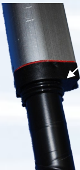
It leaks here, so we added the O-rings and coated the whole actuator in plastic sealant.
