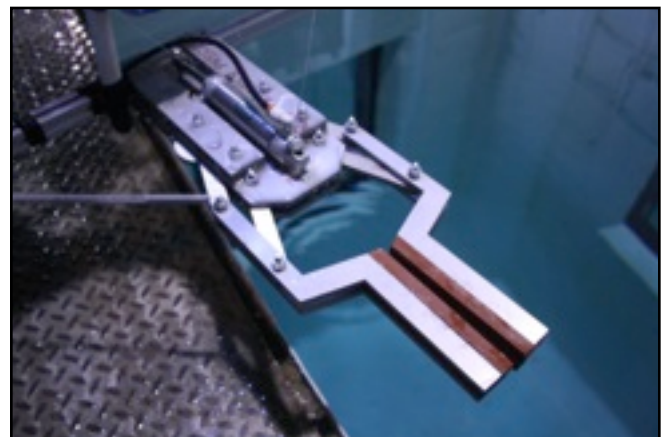
Figure 4 - The pneumatically controlled gripper
