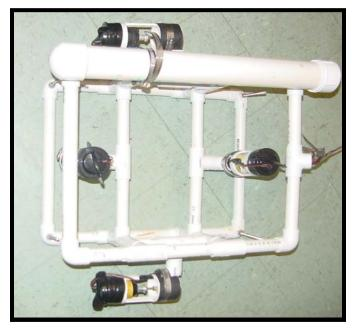
The ROV has four propellers for thrust. Two propellers make the robot go forward, backwards, left and right. The other two make it go up and down. These propellers allow the driver to control the movement of the ROV in a practical, easy way.
