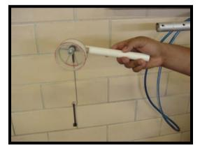
The ROV uses a sensor to detect metal material on the debris field. The device uses a magnet attached to a rod that pivots on a bolt. We can determine if the object is metal by simply seeing how much the sensor is attracted to the object. There are lines pre-drawn so that we can see the max height the rod reaches.
