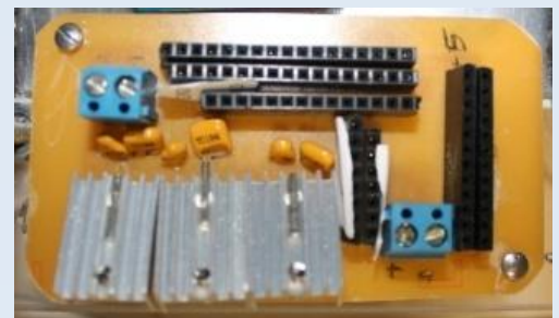
Fig.16 – Voltage Regulator board (12V, 10V, 6V, 5V, GND).
