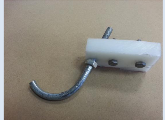
Fig.23- Hook used in Maximilian ROV.
