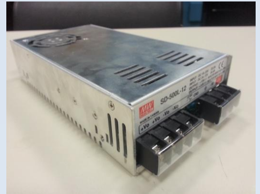
Fig.14 –DC/DC converter used.
