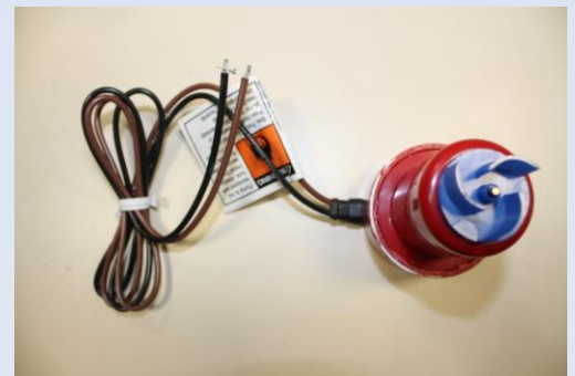
Fig.7 - Bilge Pump before modification.
