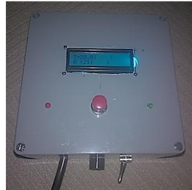
Figure 19: The temperature sensor control box
