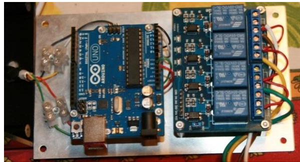
Arduino with payload control relays
