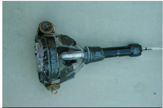
Temperature probe with field developed alignment basket
