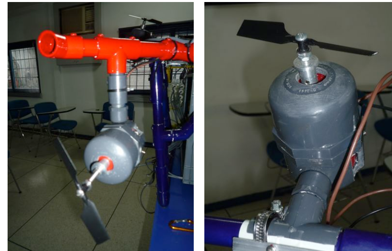
Figure 11. Horizontal thruster covert (left). Vertical thruster covert (right). R.M.
