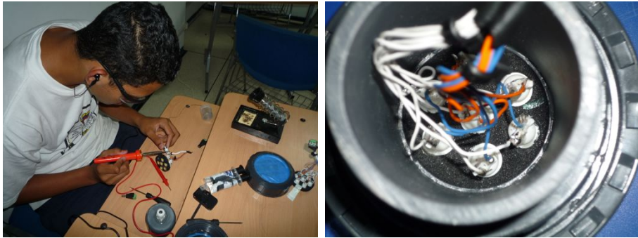
Figure 15. Pilot Macgregori Briceño soldering the LEDs array. (left). Inside view of the LEDs array embed in black expanded rubber (right). R.M.
