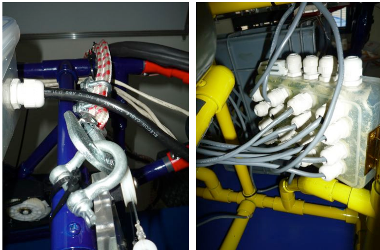
Figure 23. Tether security hook attached to the back of the blue section (left). Junction box inlets, outlets and door hinge. R.M.
