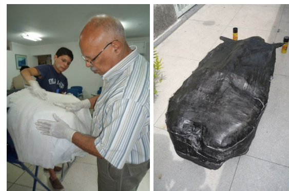
Figure 9. Left, applying the plaster badges to the ROV structure to create the mold. Right, ROV fiberglass fairing. R.M.
