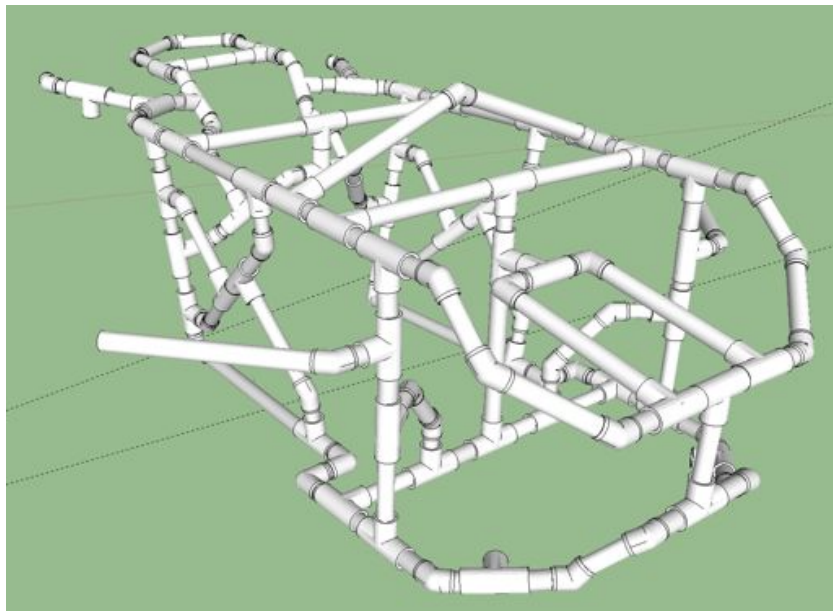
Figure 7. CAD structural design in Google Sketch Up 8. Truss implementation is evident in Tricolor Turtle RS-01 structure. R.M.
