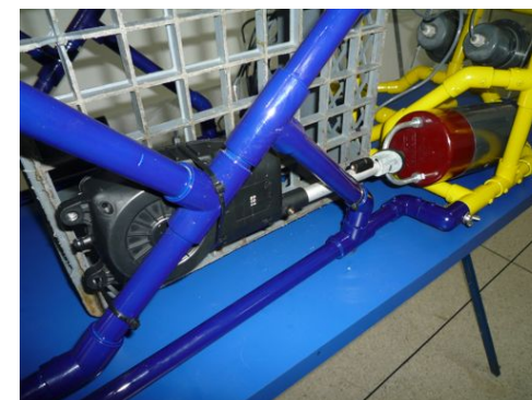
Figure 19. ADCP retrieval system. All deployment and retrieval systems are located within the blue section (middle) of the vehicle. R.M.
