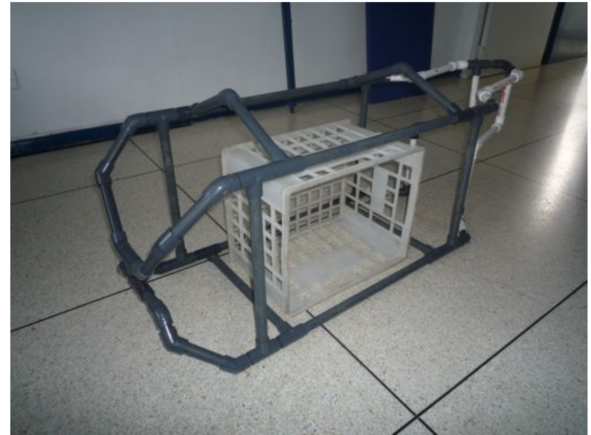
Figure 6. First PVC prototype of the ROV Tricolor Turtle RS-01. The structure was built around the SIA. R. M.
