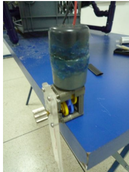
Figure 16. Robotic Claw MKII and extension boom (left). Gear box modification and motor assembly (right). R.M.
