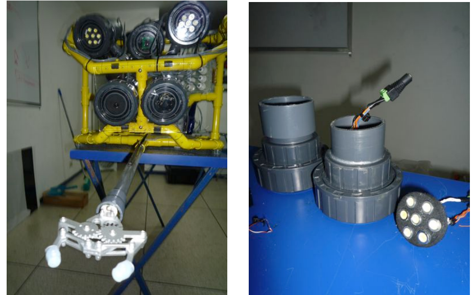
Figure 14. Left, vehicle front cameras and lights. Right, pressure housing and LEDs array. R.M.
