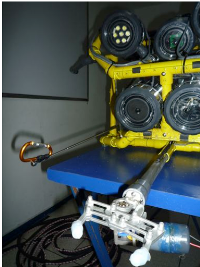
Figure 16. Robotic Claw MKII and extension boom (left). Gear box modification and motor assembly (right). R.M.
