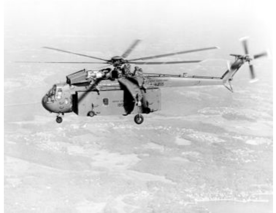
Figure 2. The Sikorsky CH-54 Tarhe is a twin-engine heavy-lift helicopter designed by Sikorsky Aircraft for the United States Army. Wikimedia Commons.
