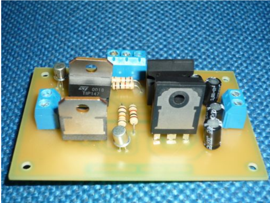
Figure 20. 10 A H-bridge motor controller PCB from PyroElectro.com. R.M.
