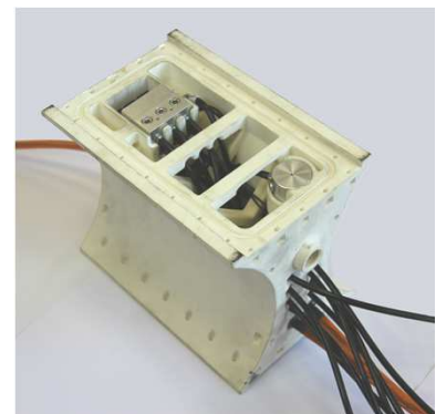
Fig. 1.7 The hydraulic system pressure hull
