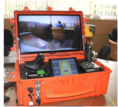
Fig. 5.1 Shore Control Station
