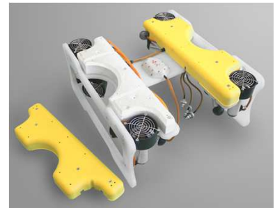
Fig. 1.2 The Akvator-3D buoyancy and frame
