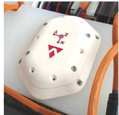
Fig. 2.8 Pressure hull of the orientation sensor
