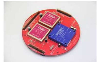
Fig. 2.2 Power supply board
