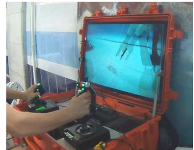
Fig. 3.1 Shore control station
