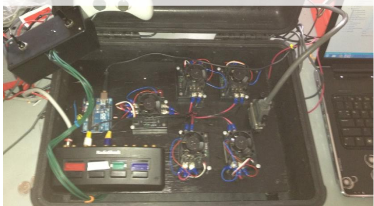
Figure 11: Completed Control System: Arduino, Motor Controllers, Camera feed, Switches
