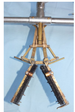
Fig 1.8 Rovbotnica's custom-built manipulator
