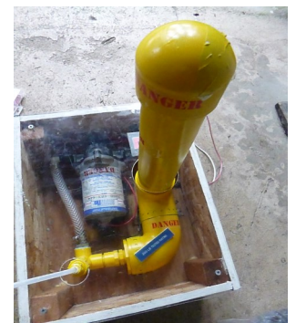
Fig 1.1.3 Hydraulic pressure accumulator
