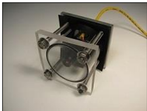
Figure 1-10: One of the maintenance-free camera canisters.
