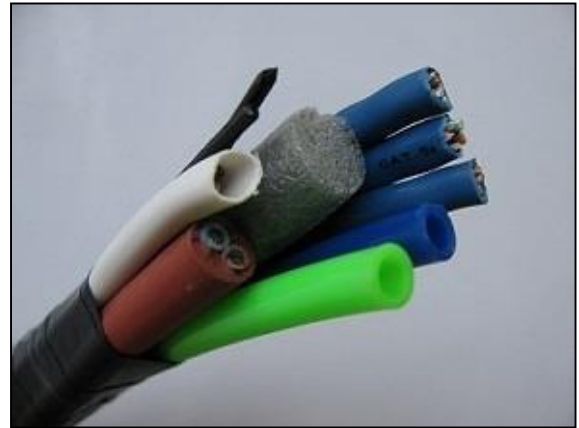
Figure 1-12: A cross section of the complete tether.
