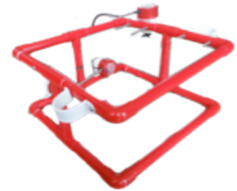
The design concept (left) and product: the bare chassis of the ROV. Note the one unsupported edge and simple shape.
