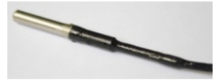
A bare DS18B20 thermometer without its PVC mounting.
