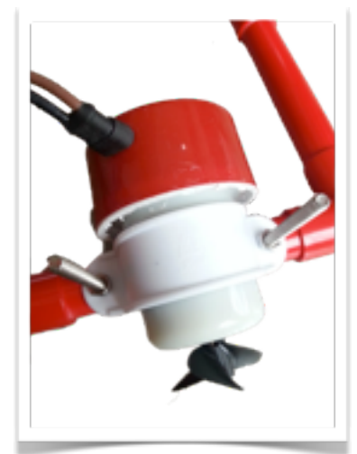
A secured bilge pump with pump component removed and (exposed) propellor fixed to a pipe
