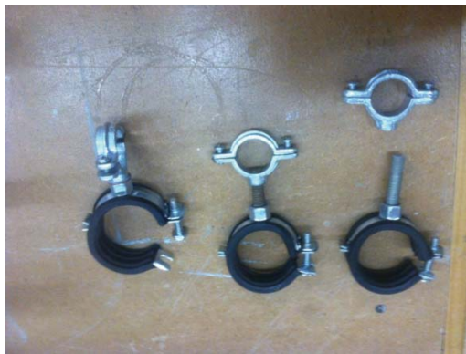
Threaded rod, metal and rubber split rings were used to secure the thruster motors
