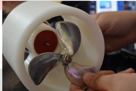
Fig 8: Setting up propeller with coupling with motor.
