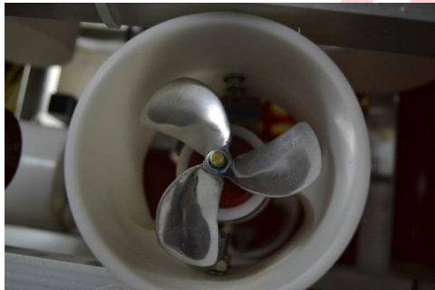
Fig 9: Propeller fixed with motor using lock nuts.
