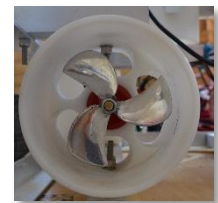
Fig 24: Kort Nozzle protecting motor and propeller.
