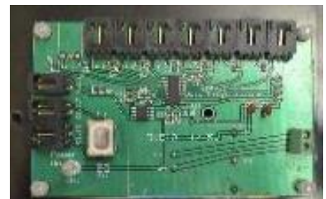
Figure 17: Video Switcher PCB
