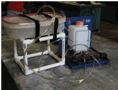
Image 7 – Ballast System Model
