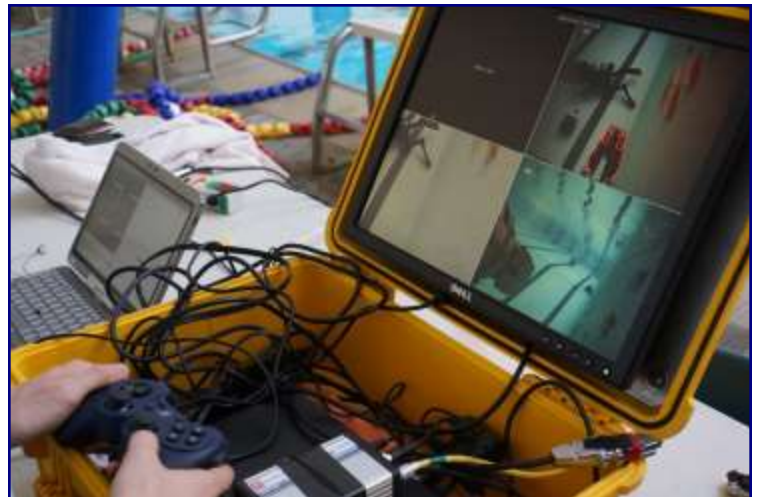
Fig 2.2 The control station with controller, DVR screen, and laptop screen.
