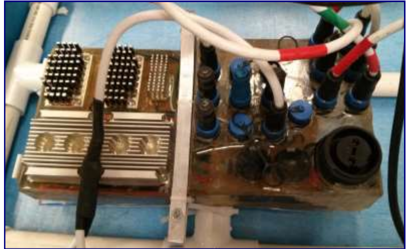
Fig 3.2 The DC-to-DC power brick.
