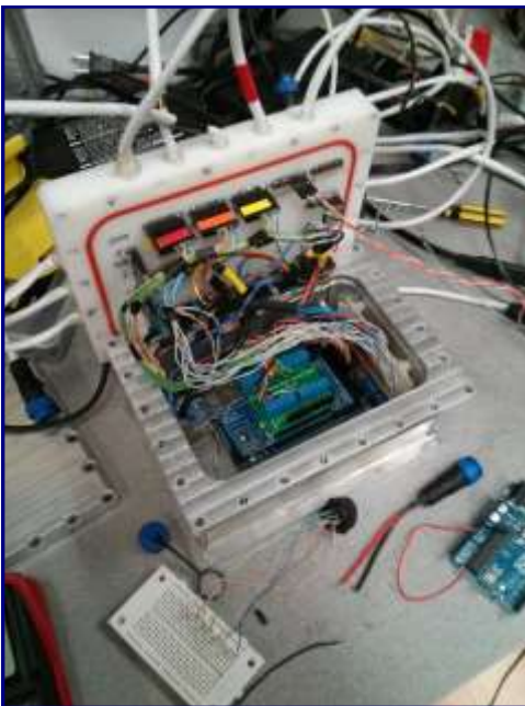
Fig 2.1.B Arduino and Ethernet shield inside Pressure Housing
