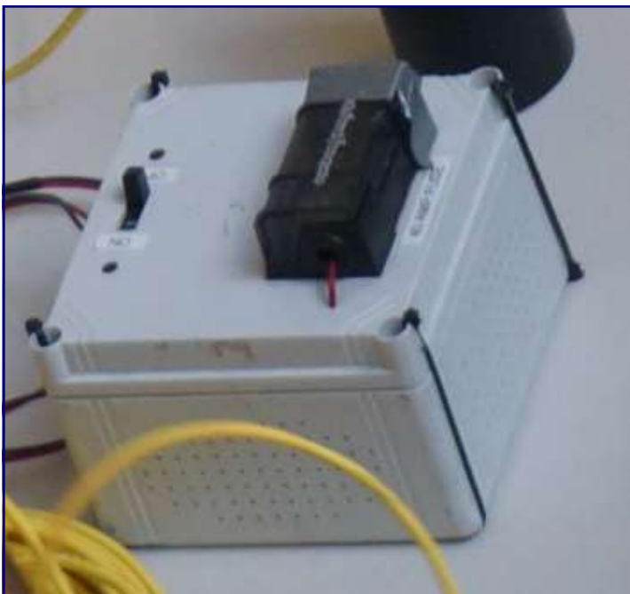
LBCC 40A Fuse and Safety On/Off (to be plugged into MATE T.S. 48VDC Power Supply)
