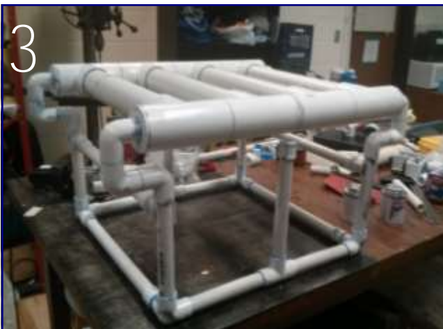
Fig 1.1.3 Reduced length and width of the ROV. Top buoyant section too long to connect to bottom, necessitating awkward joints at the top corners, causing increased cost and reduced structural integrity.
