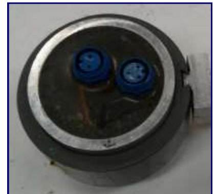
Fig 1.3.2 (bottom) Aluminum and epoxy camera housing
