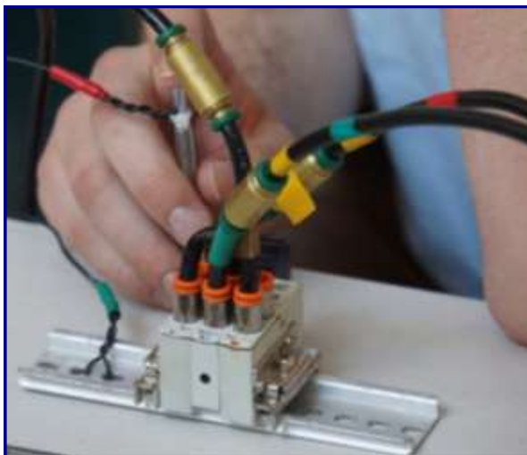
Fig 2.2.D Solenoid switch for pneumatics
