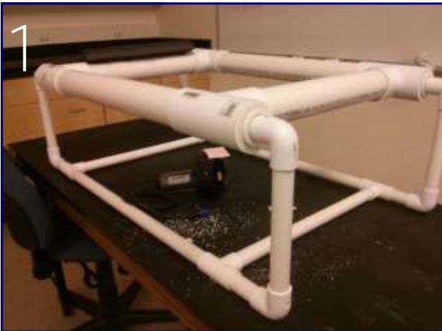
Fig 1.1.1 2" PVC tubing on top for main buoyancy, 3/4" tubing for bottom structure. Smaller than previous year's frame.
