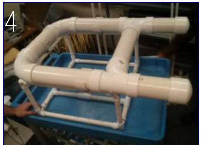
Fig 1.1.4 Open top facilitates access to internal systems. Top buoyancy tubes increased from 2" to 3" PVC pipes. Increased buoyancy by 5.7L of air, even after the removal of top cross tubes
