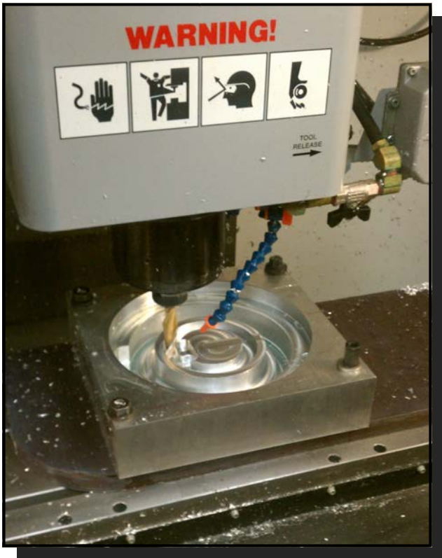
Team members machining end cap from a block of aluminum
