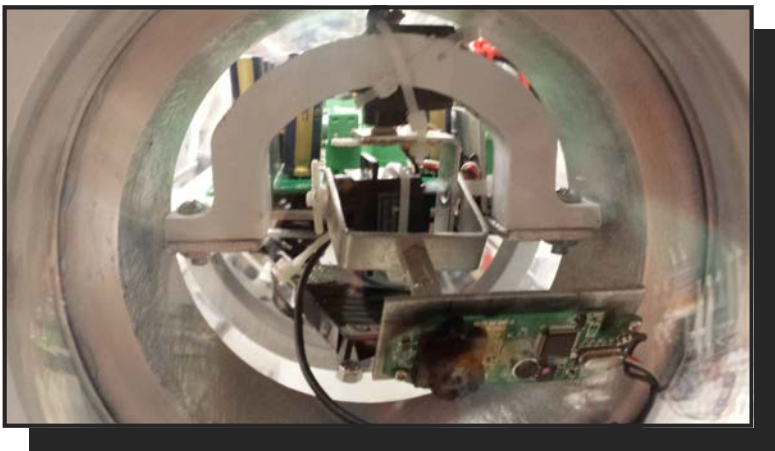
Logitech C110 camera removed from its plastic housing and mounted to a pan and tilt system
