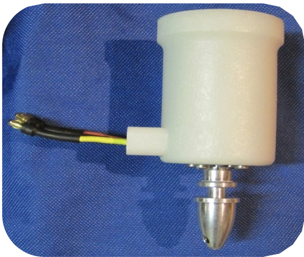
Figure 7—Custom Motor Housing
