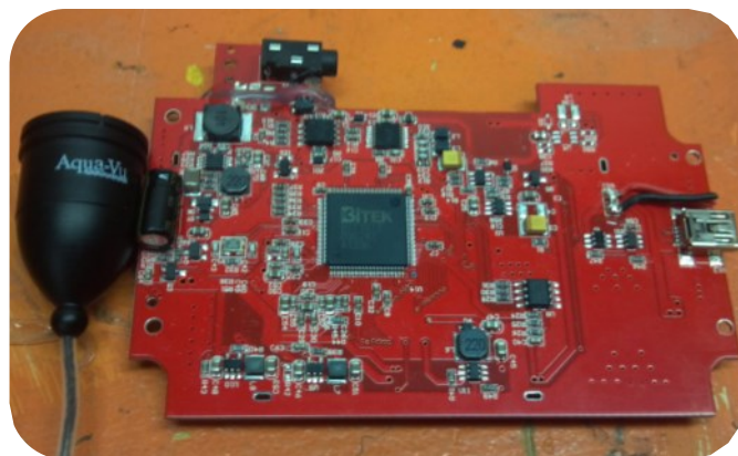
Figure 13—Aqua-Vu camera next to its processing board
