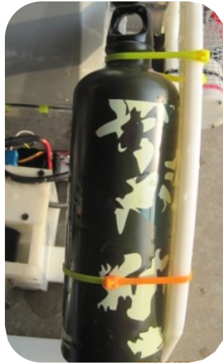
Figure 17—Aluminum water bottle attached to Bubbles ' frame
