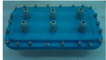
Fig.13: Payload Electrical container.
