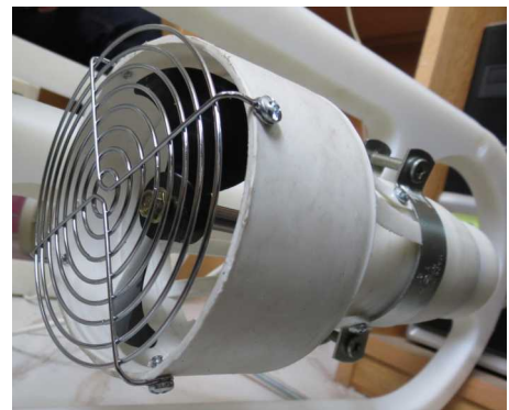
Fig.6: Side view of a mounted thruster.
