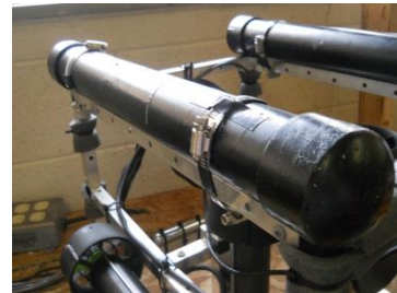
Buoyancy Tubes of TRITON
