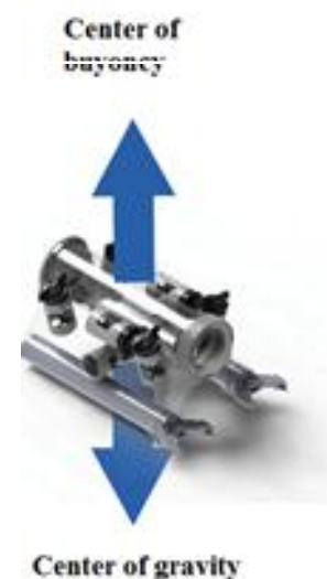
Fig.10: Centers of buoyancy and gravity
