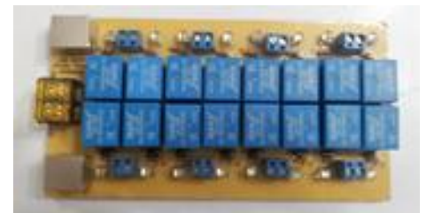
Fig. 23: Board of relays.
