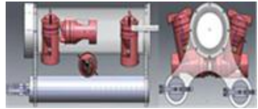
Fig. 5: Triton's thrusters' arrangement.
