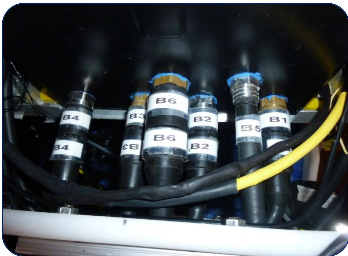
Figure 6: The SubConn bulkhead connectors drilled into the dry housing
