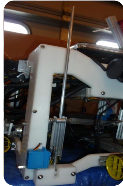
Figure 14: The aluminum rod gripper used to extract the ADCP from the mooring platform
