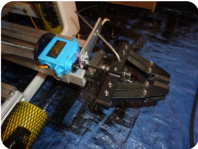
Figure 13: Nemo's clamp gripper with the ability to move up and down, as well as rotate 100 degrees
