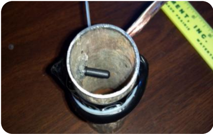
Figure 16: A simple temperature sensor constructed of a 15 cm piece of galvanized pipe
