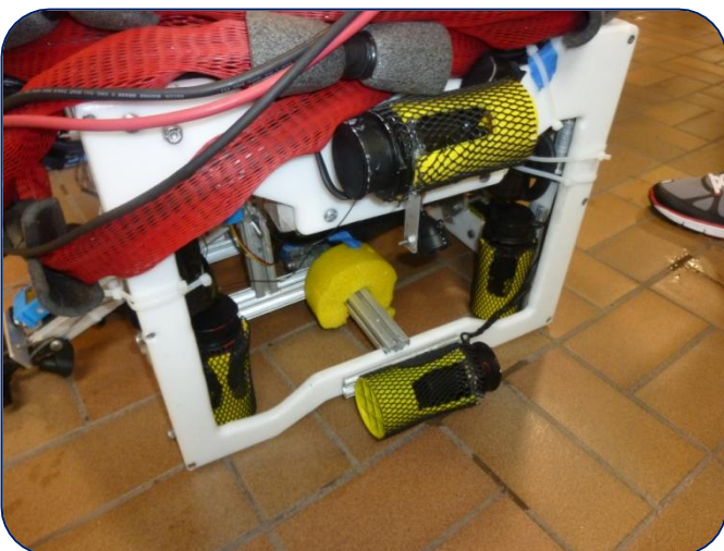
Figure 7: A side view of the Tsunami 1200/ Octura 1250 propeller setup
