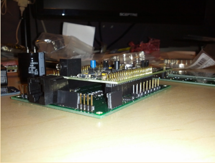
Fig. 12 - The main board resting on the microcontroller adaptor board.
