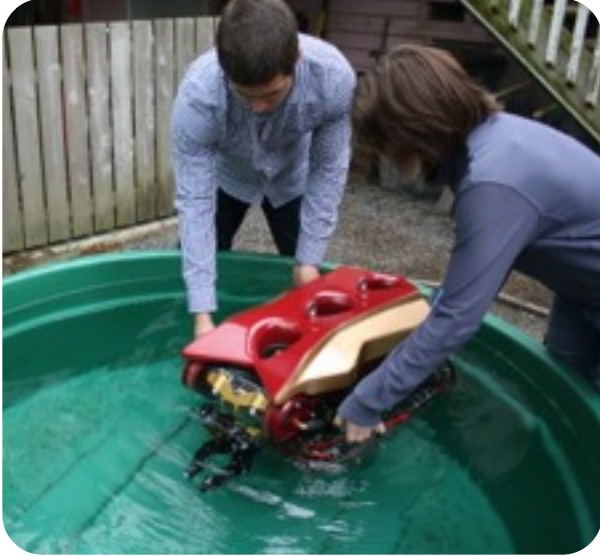
Figure 8 - Stanley Janicki and Madison Walkup testing Project ΣVI for buoyancy
