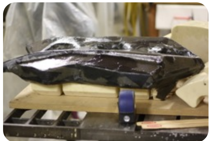
Figure 3 - Polyurethane float in the process of being coated in carbon fiber
