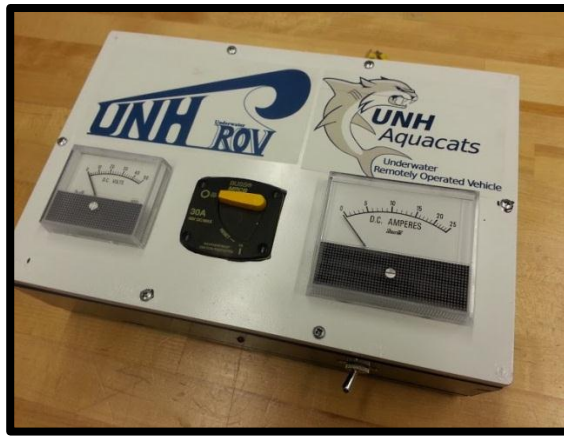
Figure 8: Fuse Box with switch, ammeter, and voltmeter.
