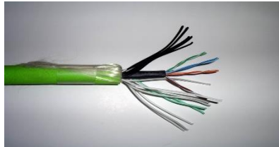
Figure 7: Outland C-3400 Tether conductors, rated for 300 volts, to transmit the DC voltage to the ROV along with one Cat5e Lan Cable (4 TP #24 AWG) for communications.
