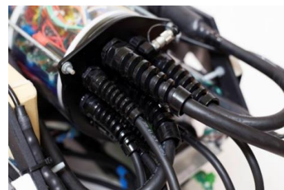
Heyco cable glands help create waterproof seals around the connectors (credit: D. Diblik)
