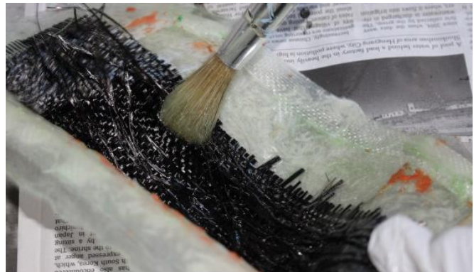
Making the carbon composite layup (credit: A. Miller)
