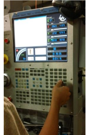
Operating a CNC machine (credit: C. Orndorff)
