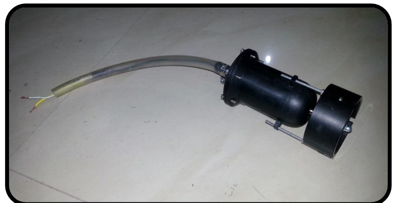
Fig 11 wire sealing with hose and jubilee clips
