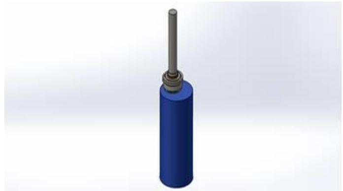
FIGURE 17 - ACTUATOR WITH POWER SCREW
