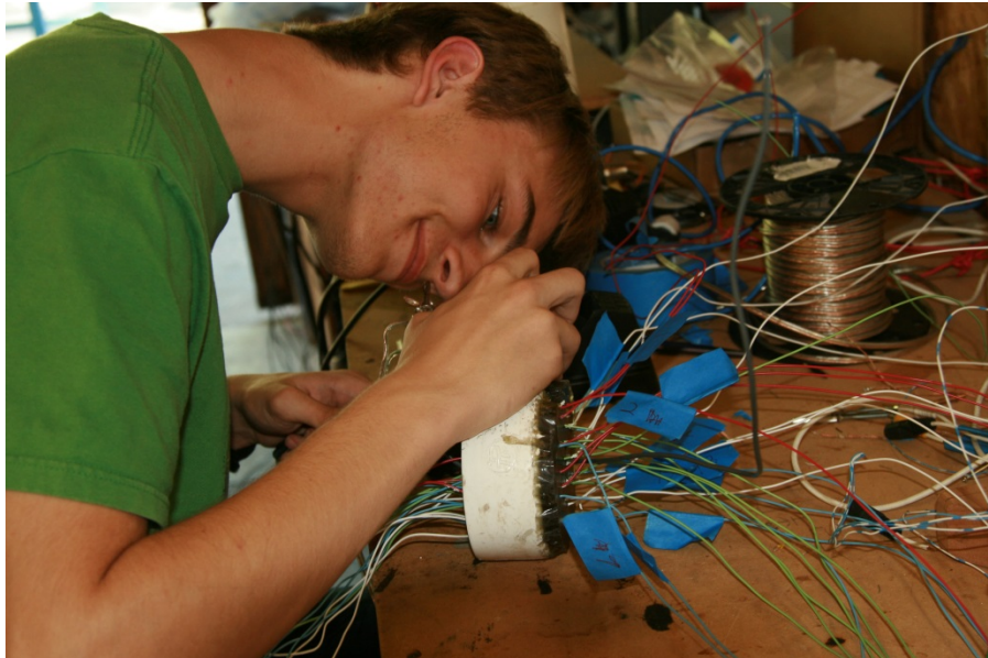
Assembling the water-proof signal housing cap
