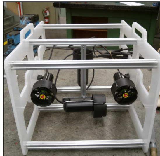
Figure 3. Aluminum T-slot cross members with thrusters installed
