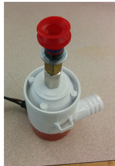
Figure 11. Suction gripper for hard to grab objects
