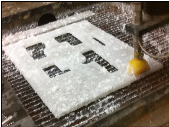
Figure 2. Polyethylene side panel being cut to shape on a water jet cutter
