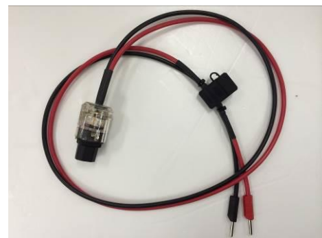
Figure 27: 20-Amp fuse to prevent overloading of power
