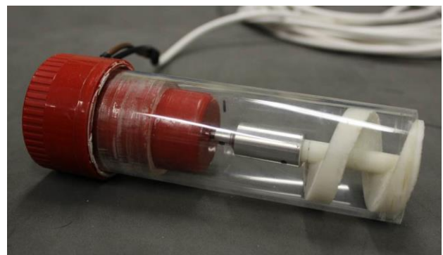
Figure 24: A screw-like retriever for the task of retrieving samples of a microbial mat
