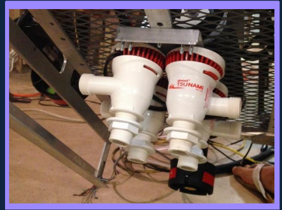
Bilge pump system used for vacuum manipulator
