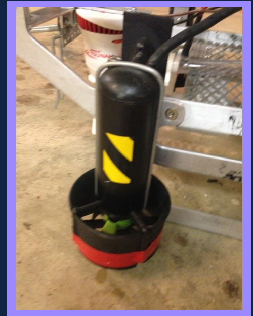
Vertical Thruster with safety precautions
