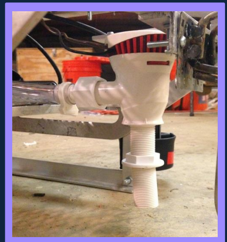
Modified bilge pump to collect agar
