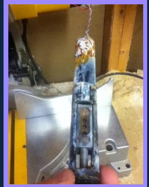
Corroded Seabotix Claw
