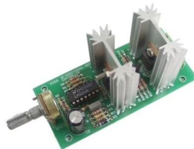
Figure 21: K-166 Motor Controller. (A. Short, 2014) Uses Pulse PWM to maintain motor torque. Max. 32VDC operation for controller. IRFZ44 Mosfets can handle up to a maximum 49amp.
