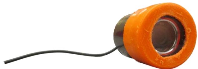
Figure 28: Custom Rear Camera. (A. Short, 2014) The Jetview camera with its custom-designed case offers a view from the rear of the ROV.
