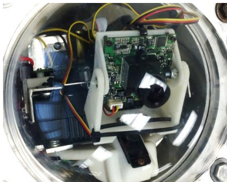
Figure 3: Pan and Tilt Camera inside acrylic dome with custom 3D printed mount
