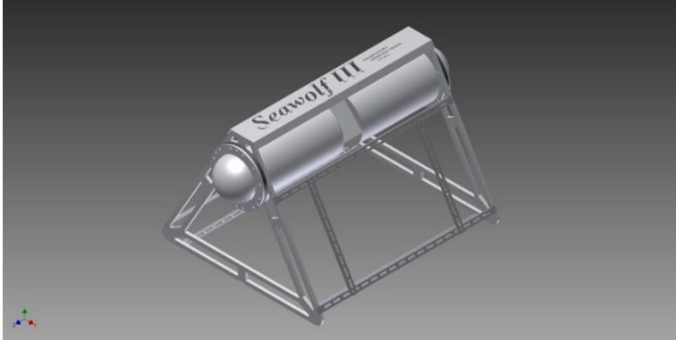
Figure 2: This is a 3D rendering of the frame and main electronics housing minus the outriggers that hold the buoyancy compensating tubes.
