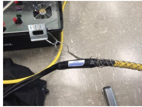
Figure 17: Showing one side of the strain relief hooked to the power supply
