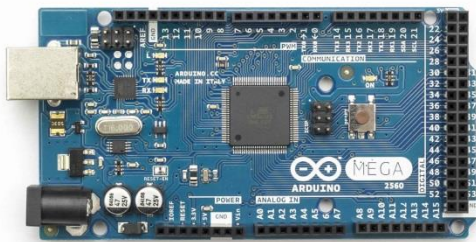
Figure 9: The Arduino Mega microcontroller was used last year for the control system
