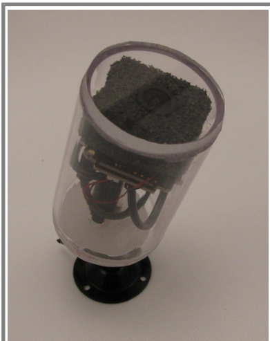
Figure 21: An outer camera, kept waterproof by the canister.
