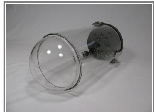
Figure 5: The waterproof canister that contains the electronics and pneumatic manifold.
