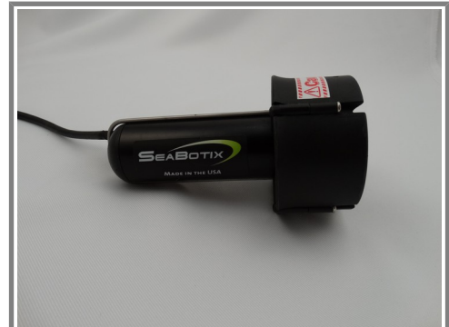
Figure 6: A Seabotix thruster. These supply the majority of the thrust for the Hydrus.
