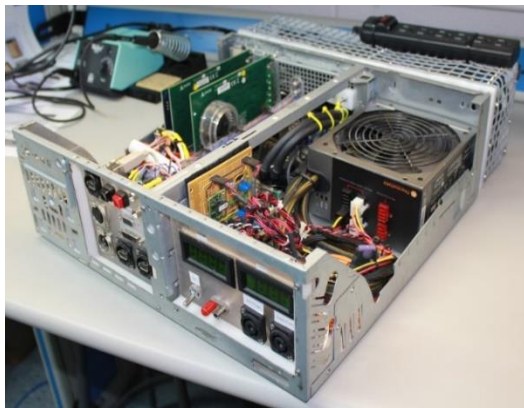
Figure 4. Topsides Control Module
