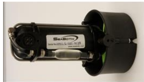
Figure 3. SeaBotix® HPDC1502 brushless thruster
