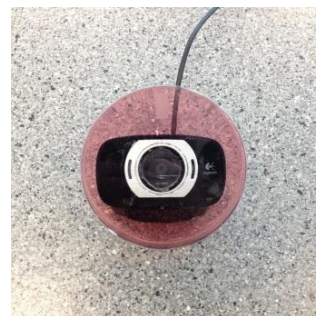
Figure 5: The HD Webcam potted using epoxy for waterproofing
