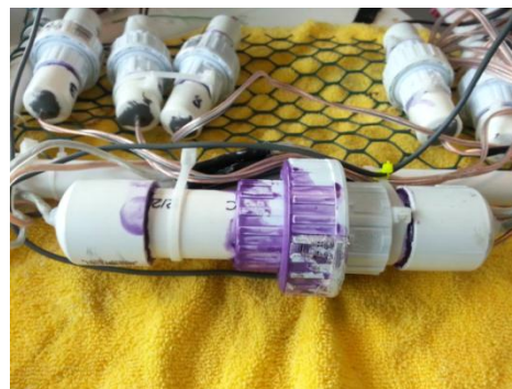
Figure 3: The PVC union system allowing for modular connections between ROV components and the power source
