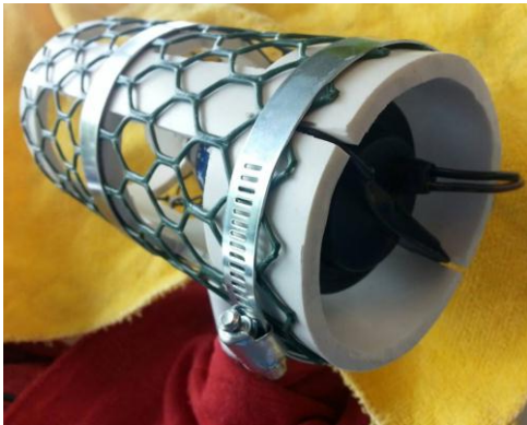
(Photo 2: Thruster in newly designed shroud)
