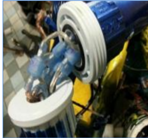
Photo 7: Team-designed PVC union “quick connects” for tether connection (large) and tool packages (small)
