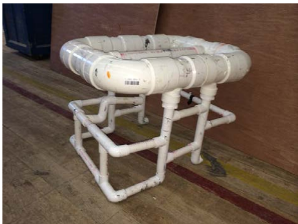
Early frame design. Bulky, cracked during testing.
